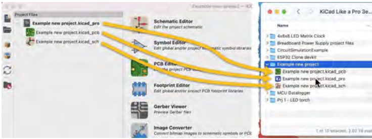
Figure 2.5.3: The new project is ready.
