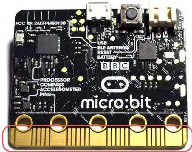
Figure 5.3.10.1: Gold fingers on a Micro:bit.
