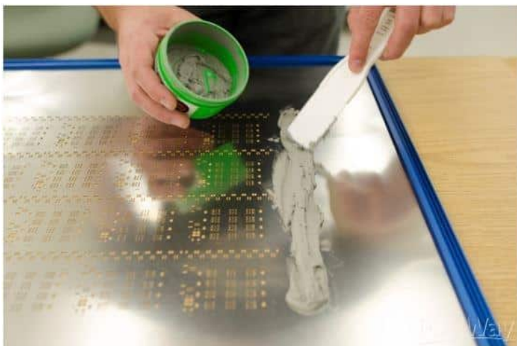
Figure 5.3.13.4: A stencil, with solder paste being applied using a squeegee (photo courtesy of Pcbnew.com).
