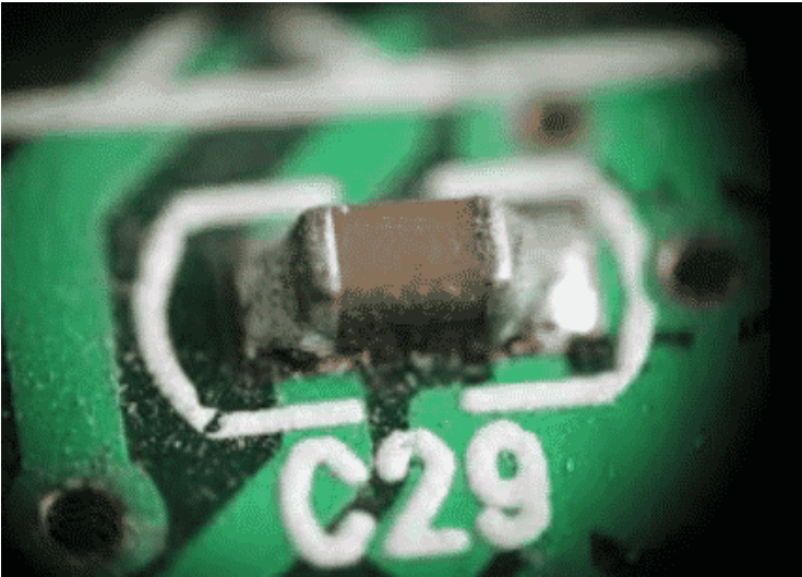
Figure 1.1.3: A surface-mounted component attached to a PCB.
