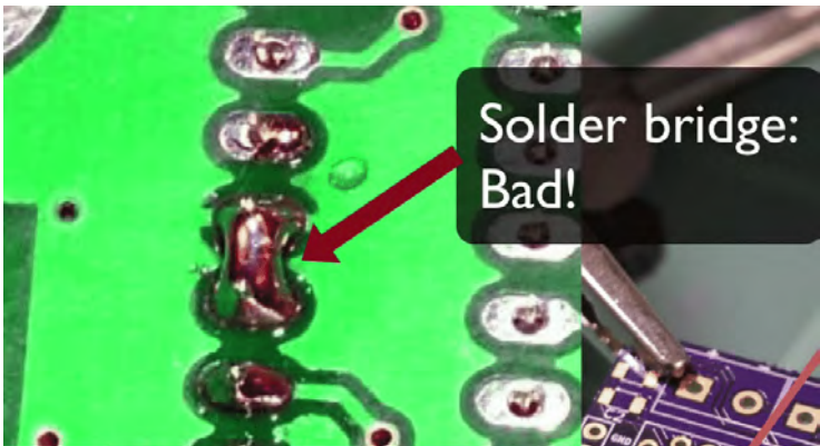
Figure 1.1.6: A solder bridge like this one is a defect that a solder mask can prevent.
