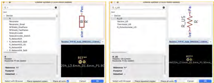
5.2.2: A resistor, European-style (left) and American-style (right).
