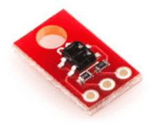
An infrared line sensor is a simple device made up of an infrared emitting LED and an infrared sensitive photo-resistor.
