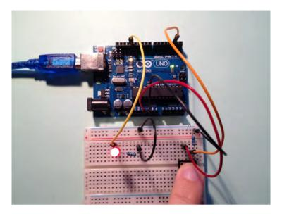
The button circuit on a breadboard.
