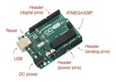
The most important features of the Arduino Uno board
