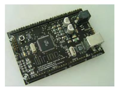
Hernando Barragán's Wiring Board, the Arduino's predecessor (original image available at https://arduinohistory.github.io/)
