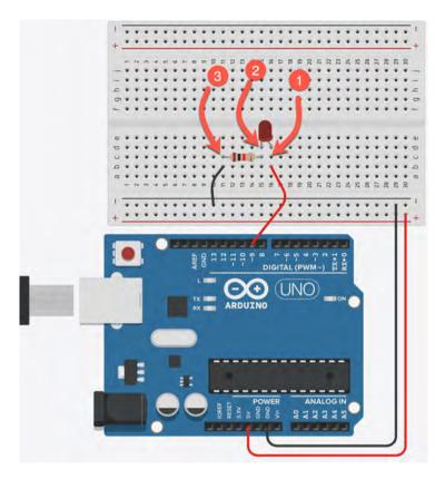
The wiring diagram for the "blinking LED" experiment.
