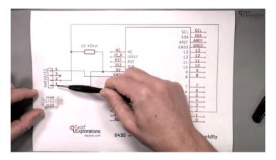
Pin number one is located on the leftmost end of the sensor, while pin number four is on the rightmost end. In some cases, you may come across DHT22 sensors with only three pins. These are typically sold as part of a breakout for the sensor. In these cases, the number three pin is left unconnected. You can simply push it up and set it aside.
