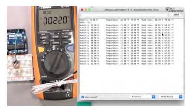
Testing the accuracy of the DHT22 with a multimeter
