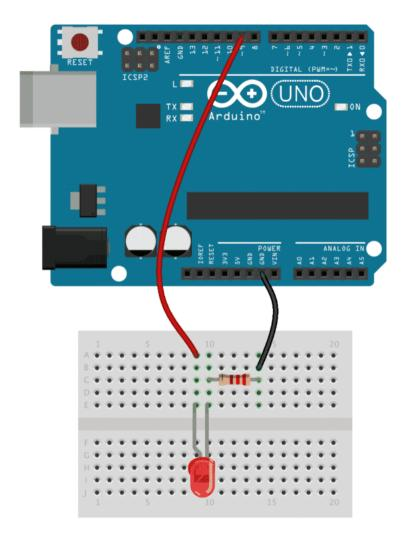
An LED is connected to digital pin 9. A 220 resistor protects the LED from too much current flowing through it.
