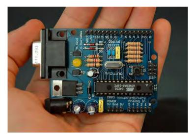
An early Arduino. It uses the RS232 serial interface instead of USB, an ATMEGA8, and male pin headers instead of female. The large black chip at the bottom right of the board is the microcontroller.
