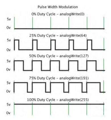
PWM and duty cycles (original: arduino.cc)
