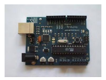
The second Arduino prototype (original image available at https://arduinohistory.github.io/)
