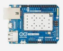
The Arduino Yún, geared for the Internet-of-Things applications (image taken from arduino.cc)
