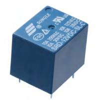
A relay is used to drive large loads from your Arduino.
