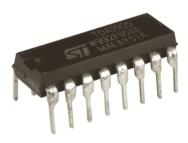
A shift register IC makes it possible to control many digital components with a single pin of your Arduino.
