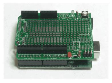
A prototyping shield has enough space and pads where you can attach your own components.
