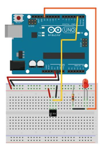
This circuit will detect motion through the sensor, and send a signal to the Arduino via digital pin 2. The Arduino will receive the signal and in turn activate the LED via digital PIN 13.
