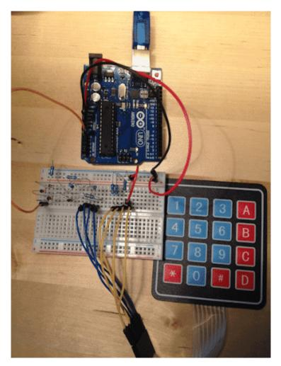
Using a  $4 \times 4$  keypad requires external wires, diodes, and resistors; this is more work (compared to a shield), but often the flexibility you get in return is worth the effort.
