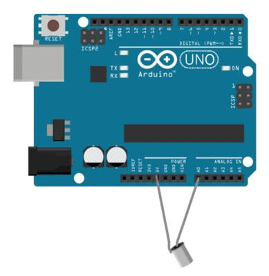
Connect one wire to 5V and the other wire to A0 analog pin
