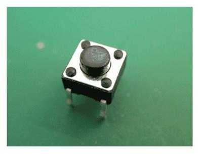
A button like this one is a digital device. Connect it to a digital pin.
