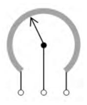
A variable resistor, like the one inside a potentiometer.
