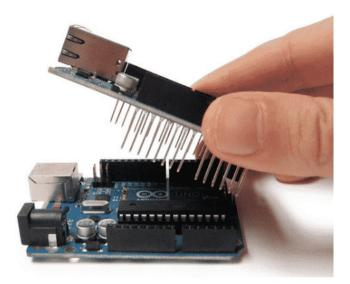
An example Arduino Uno shield. It fits perfectly in the Arduino Uno headers and adds capabilities without any jumper wires.
