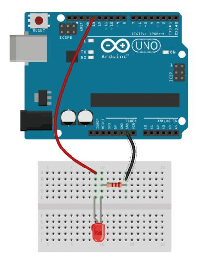
An LED is connected to digital pin 13. A 220 resistor protects the LED from too much current flowing through it.
