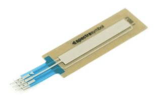
A membrane potentiometer. Electrically it works like a normal rotary potentiometer.
