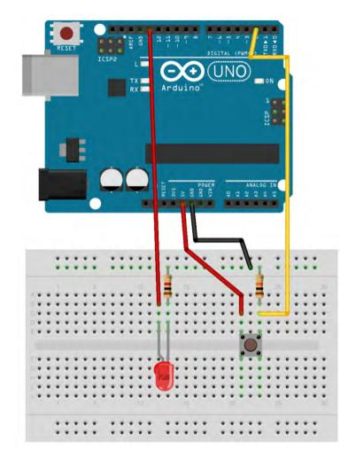
A simple button circuit. When you press the button, the LED turns on.
