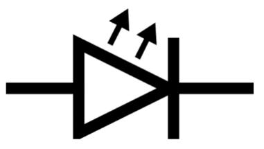
The schematic symbol for an LED
