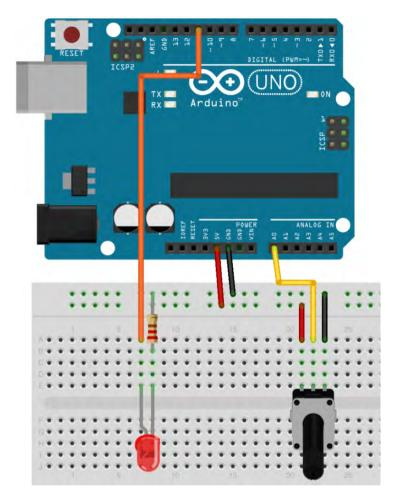
This circuit uses a potentiometer to control the brightness of an LED.
