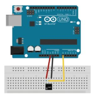
The completed circuit of the Arduino with an QRE1113 infrared line sensor
