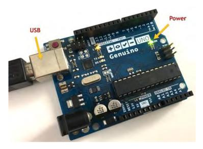
The Arduino is connected to your computer via a USB cable, and the power LED is lit
