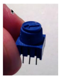
A potentiometer is a very simple sensor. It senses the position of its knob.
