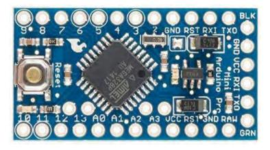
The tiny Arduino Pro Mini (image taken from arduino.cc)
