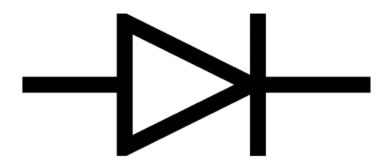
The schematic symbol for a regular LED
