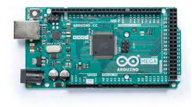
The Arduino Mega 2560 (image taken from arduino.cc)
